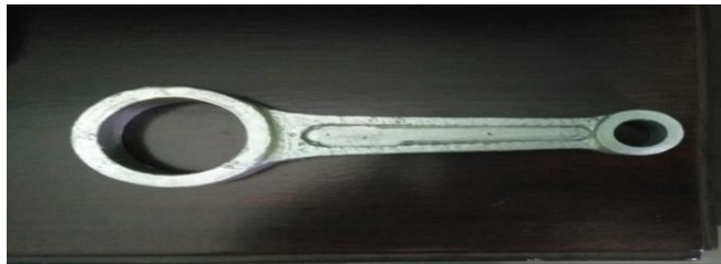
Fig. 9: Image of casted connecting rod after machining operation
