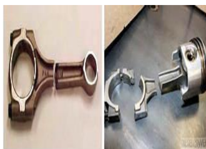
Fig.2 : Failure of a Connecting Rod
